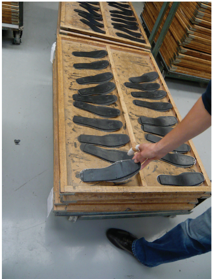
Steel-reinforced uncured rubber soles ready for use in the mold.
