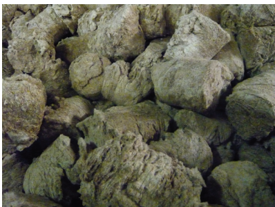
The heavier debris (sand gravel, small pieces of wood) is pressed in tablets destined to incineration.
